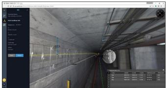
Metrorail LiDAR display showing cable placement and data extraction tool.
